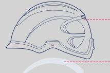
**Layer 1:** The Shell, to dissipate the impact energy.
