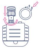
Attach the hose to the headpiece by pushing and rotating hose until it locks in position.
