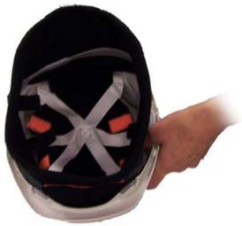
Step 3: Finally, attach the four velcro tabs that are on each side of the central cradle strap (two each side of the helmet), so that the top and bottom parts of the liner are attached together. The liner can be tucked behind the four headband retainer tabs for neatness, whilst allowing the headband to be adjusted.
