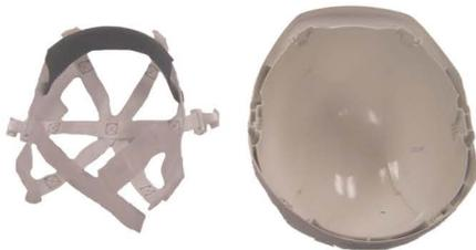
Step 1: Firstly remove the Cradle Headband Assembly. To do this, carefully push the six White kit brackets (held at the end of the webbing) out of the helmet shell.
