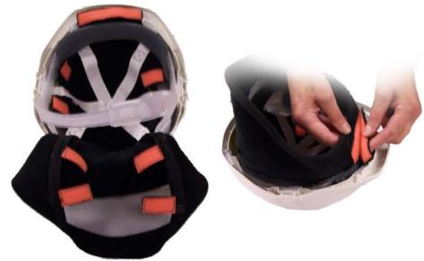
Step 2: Then while holding the top section, ensuring that the Centurion logo is facing outwards and at the back of the helmet, insert the top section into the helmet, between the back two cradle straps and the shell. With the top section under the three cradle straps, position the bottom/sides so that it sits around the outside of the headband.
